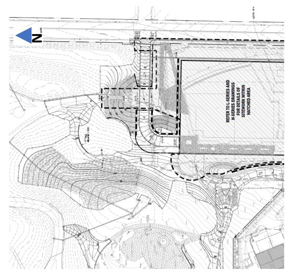
Image from page C200 of the 7/31/2017 plans showing the remaining asphalt lot and the asphalt road being added to connect the lot.
