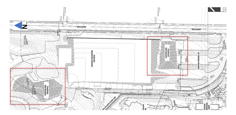
Image from page C300 of the 7/21/2017 plans showing the two existing stockpiles remaining and the regrading of the bowl (non-dashed lines are where regrading is occurring).
